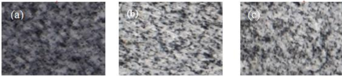
Fig 3 Plasma sprayed samples Al_2O_3 [99] @30°, 60°, 90°
